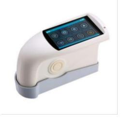
GB-NH 268 gloss meter features with 20, 60 and 85° angle, manufactured according to ISO2813 and GB/T 9754. It is also compatible with the standards of ASTM D523, ASTM D2457. GB-NH 268 conforms to JJG696 first class gloss meter working requirement, corresponding with CIE 1931(2°) under CIE C light source.
